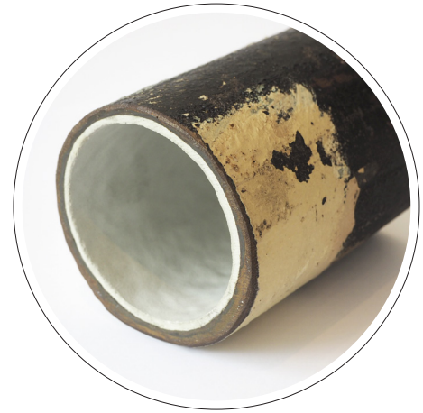
Re-lining of pipes
