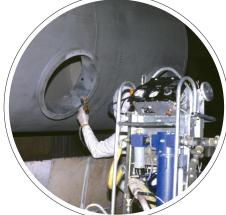
GF-8000 is in the first place intended for high viscosity resins filled with glass-flakes or other abrasive fillers. The machine can also be used for other 1- or 2-component resins such as paints, epoxy etc.
