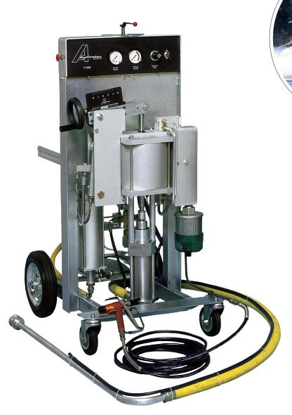
IPG-8000 is widely used and has become a best seller in the industry. The machine is a superbly designed and engineered gelcoat machine that eliminates the "bucket and brush" in hand lay up that not only minimises fumes, it will improve working conditions considerably. Using advanced and proven techniques, the machine
