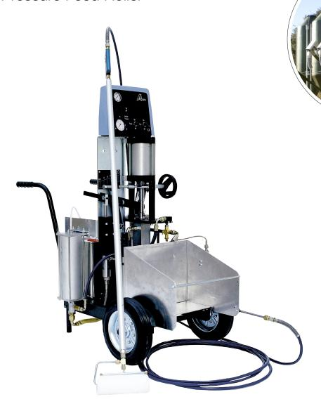
The IPL-15 Classic is a development of the now famous IPG-24/HV series and utilises proven technology from both the reliable IP-6000 series and IPG-24/HV. Components are thoroughly blended by a static mixer mounted on the machine, a pneumatically operated
