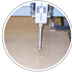
Application by mixing gun
