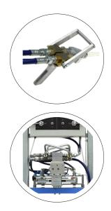
EGM T200 is, in the first place, intended for High viscosity Epoxy-resins. The equipment can also be used for other 2- component materials. The mixing ratio is continuously variable between 1:1 and 1:10. The dosing is correct to  $\pm$  1 of the adjusted ratio. Easy and reliable to handle.
