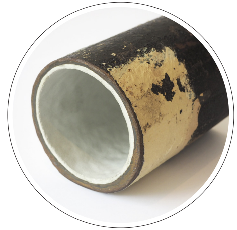
Re-lining of pipes
