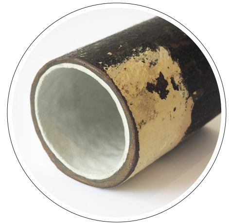
Re-lining of pipes
