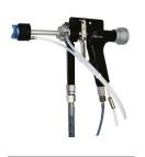
IPG-24/HV is a superbly designed and engineered gelcoater developed as a replacement for the established IP-6000 machine. It is equipped with Aplicator's patented Double Flow Technology, which guarantees accurate catalyst dosage with perfect mixing of the gelcoat and catalyst. To minimise solvent use, mixing of the
