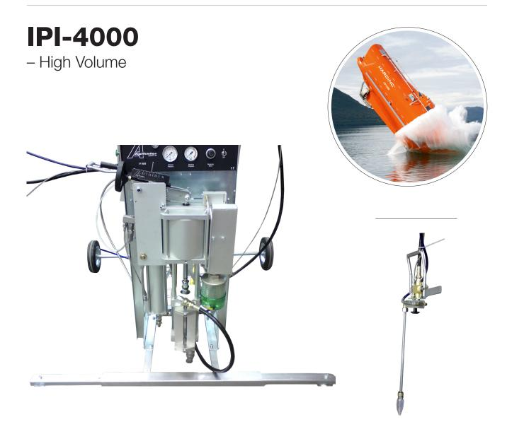
Aplicator's IPI-4000 is a superbly designed and engineered injection machine for successful Resin Transfer Moulding (RTM). Using advanced and proven techniques, the machine is easy and safe to operate with simple controls for straight forward operation. An exact resin to catalyst ratio is provided by Aplicator's unique steplessly adjustable peroxide slave pump. Internal mixing of resin and peroxide in a static mixer at the injection head, minimizes waste during flushing.
