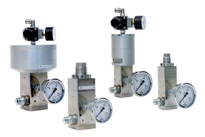
A material pressure regulator is used to regulate downstream material pressures and to minimize any pressure pulsations induced by airdriven piston pumps when dispensing viscous materials. The material pressure is easily adjusted by screw or by an air driven servo. The regulator can be adapted to highly abrasive and corrosive materials. Material pressure can be regulated in the range of 1-200 bar.
