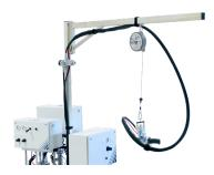
Manual system fitted with two HVP200 feeding pumps, suitable for high viscosity materials. Mixing gun fitted on a pedestal and operated with a foot pedal.
