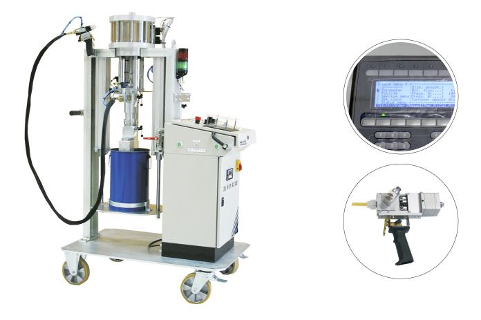
Basic specification of the 2K HVP AX is for the dispensing of two component materials or one component with injection of a booster/ accelerator as a water based paste. Typical machine is used for sealing and bonding in industries such as train, tram, bus, truck and automotive where mobility is required. Excellent for Polyurethanes, Polysulfide's, Silicones and MS polymers. 2K HVP AX can also be used as a fixed system that feeds directly from 200 kg barrels.
