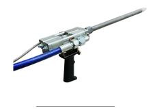
Aplicator's IPP-8000/T200 MG (mixing in gun) is designed for application of medium to high viscosity materials such as polyester putty, sealants, silicones, grease, adhesives and other similar materials in single or multi part form. Pumping and mixing to the right proportions demands a special technique when working with higher viscosity materials. This can be achieved with this machine even when pumping straight from
