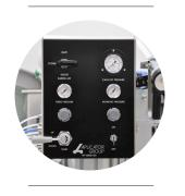
A machine specially designed for the application of medium to high viscosity materials such as polyester putty, sealants, silicones, grease, adhesives and other similar materials in single or multi part form. Pumping and mixing to the right proportions demands a special technique when working with higher viscosity materials. This can be achieved with this machine even when pumping straight
