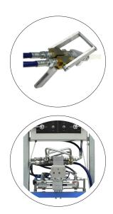
EGM T200 is, in the first place, intended for High viscosity Epoxy-resins. The equipment can also be used for other 2- component materials. The mixing ratio is continuously variable between 100:100 and 100:25. The dosing is correct to  $\pm$  1 of the adjusted ratio. Easy and reliable to handle.
